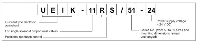
The UEIK-11RS card is an electronic control unit Eurocard type for closed loop control of single solenoid proportional valves with positional feedback control.
